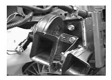
12. Use the 3/8" Whiz nut and fasten the horn to the lower bolt on the side plate.
