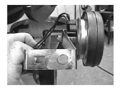
9. Remove the horn from the passenger side frame. Drill the holes to 3/8" diameter.
