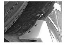
4. Remove the 7mm screws from the bumper facia/ fender well molding forward of the front tires. The two lower rivets need to be drilled out
