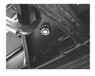
14. Drill the 1/2" holes under the metal bumper. Use the holes in the brace as a template. Use the 1/2" hardware as shown in the drawing.
